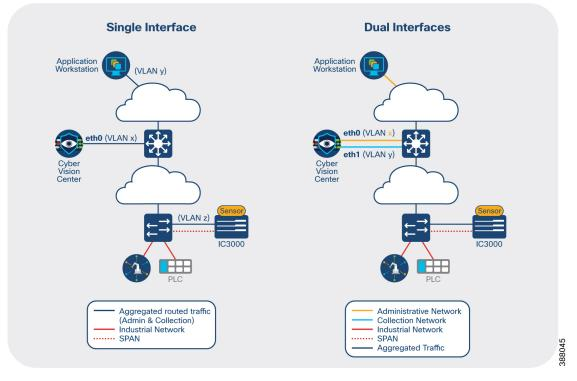
Figure 18: Cyber Vision Center Deployment Modes
