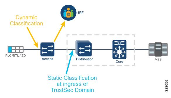
Figure 29: Static vs Dynamic Classification
