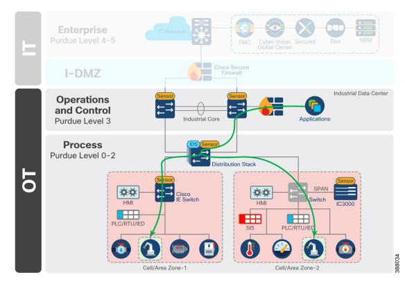
Figure 7: Applications that need access to specific services in the cell, but not the full cell
