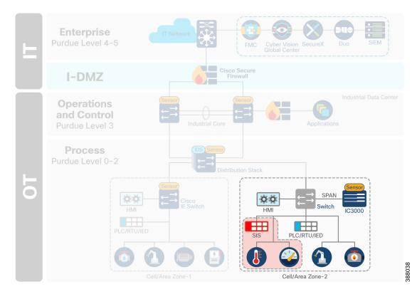
Figure 11: Safety Network could be air gapped, or logically separated from the rest of the network
