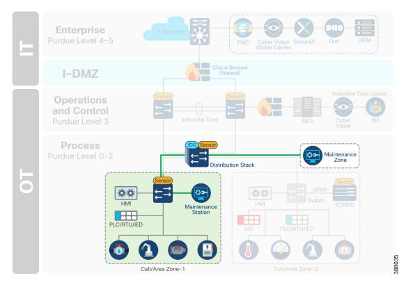
Figure 8: Maintenance workstations may reside within the cell or in a dedicated zone outside the cell
