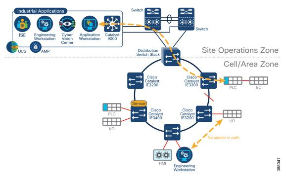
The recommendation is to always install a sensor at the top of a ring. At a minimum, all traffic leaving and entering the zone should be captured, with additional sensors placed within the ring depending on desired visibility levels.
