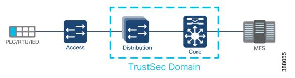
Packets entering the domain are tagged with an SGT containing the assigned security group number of the source device. This packet classification is maintained along the data path within the Cisco TrustSec domain for the purpose of applying security and other policy criteria. The final Cisco TrustSec device in the TrustSec domain, enforces an access control policy based on the security group of source device and the security group of the destination endpoint.
