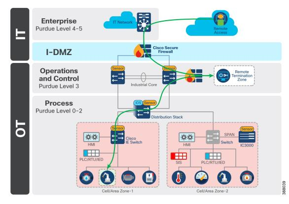
Figure 12: Remote users need access to select devices, not a full zone
