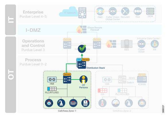
Figure 10: Operators plug into a cell using a convenience port and should be able to reach out to extra services
