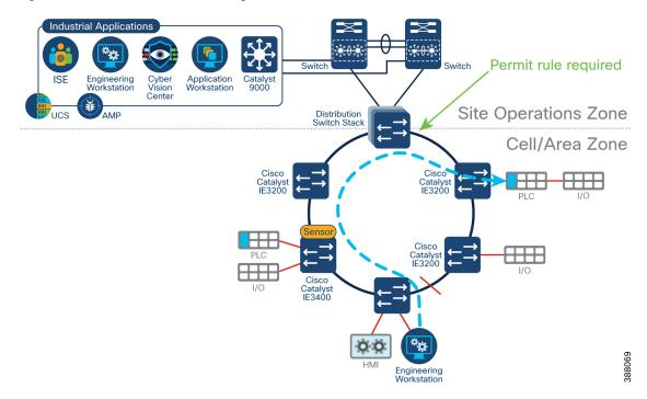
Figure 42: Inter-Cell/Area Zone traffic traversing the Distribution Switch
