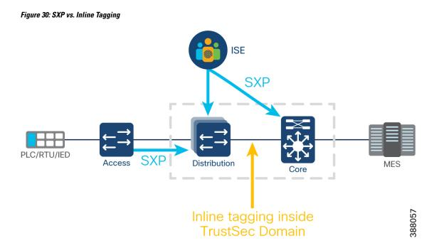
A network device performing the enforcement needs to determine the destination SGT as well as the source for applying the SGACL. The destination SGT can be determined in one of the following ways:
