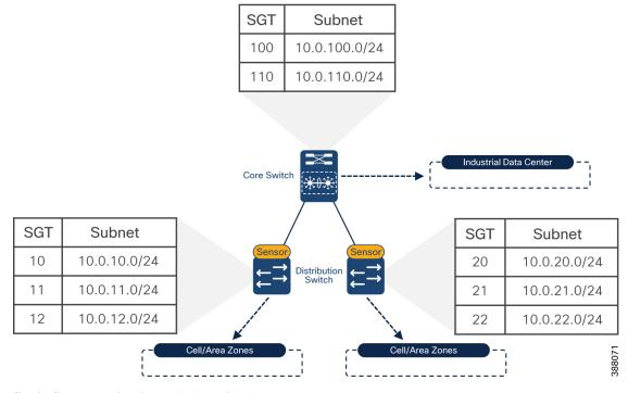
Figure 44: SXP Domain Filtering in the TrustSec Domain
