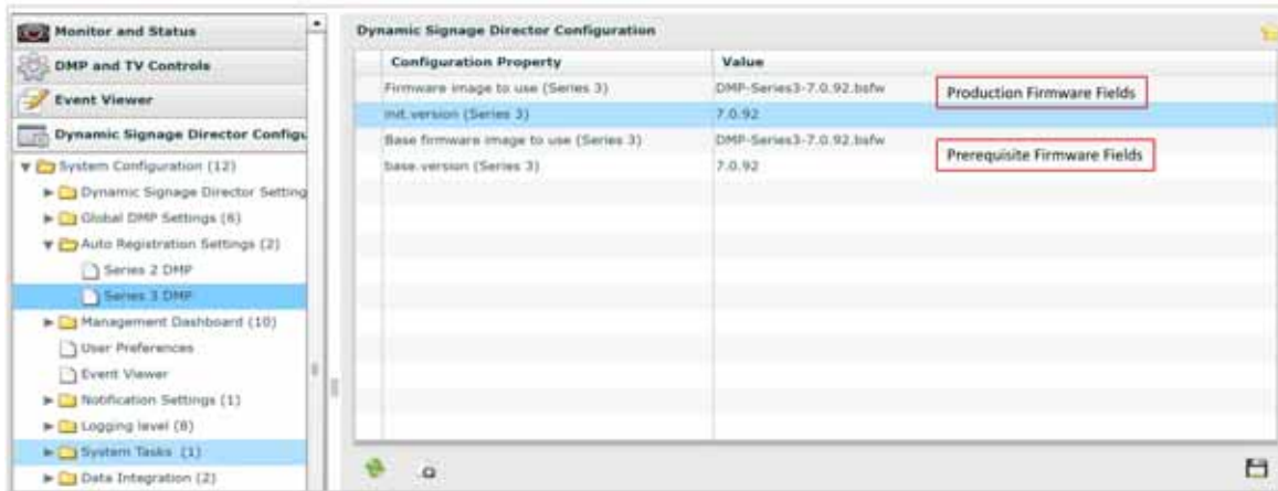
Figure 2 Firmware Image and Version Properties Required to Provision the CV-UHD and CV-HD
