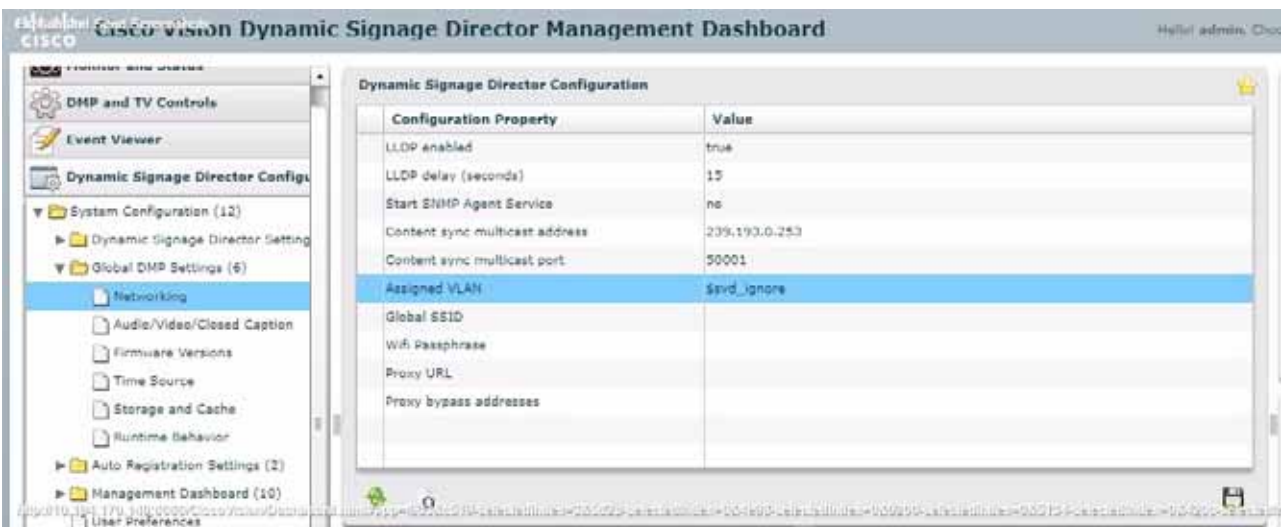
Figure 4 Assigned VLAN Property Configuration for the SV-4K and DMP-2K
