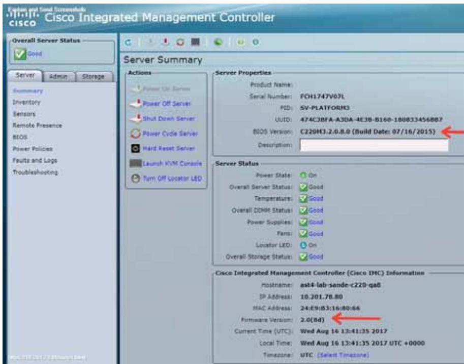
Figure 1 Firmware Verification From the CIMC Console
