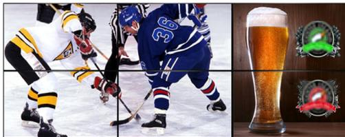
A 2x3 video wall is the most common video wall that Cisco recommends because in the left 2x2 group of displays, the game feed maintains the proper 16:9 aspect ratio of the HD game feed. This 2x3 TV/display grid can be implemented in Cisco Vision Director as two types of video walls: a 2x2 and a 2x1.
