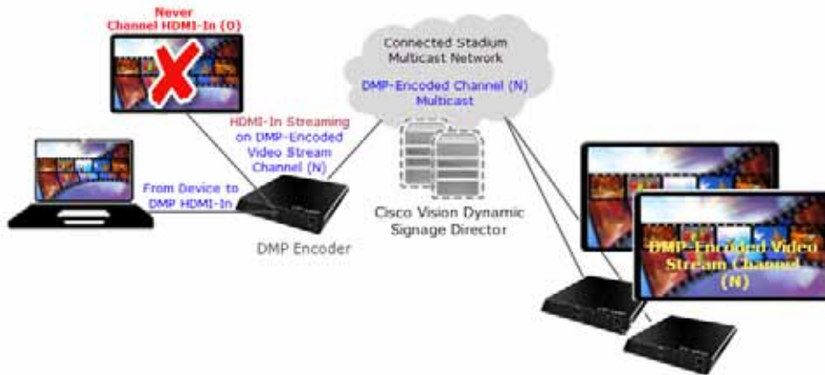
Figure 8 Unsupported DMP Encoder Configuration for HDMI-In Streaming
