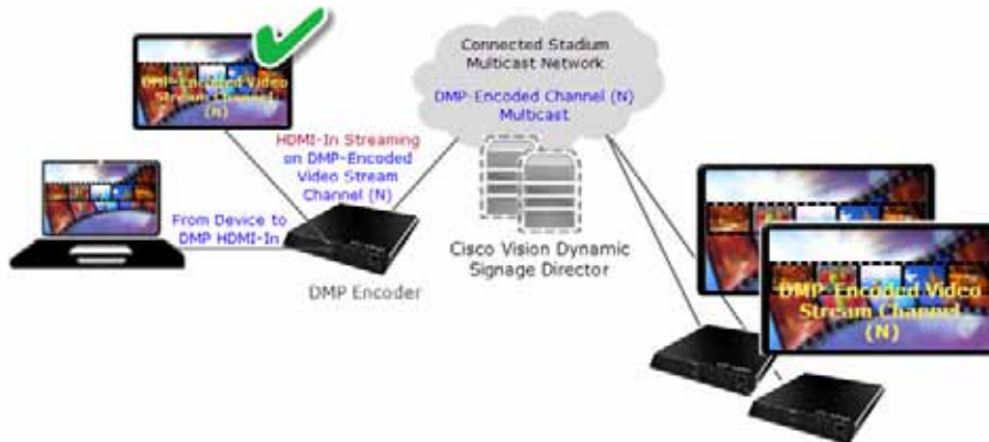
Figure 9 Supported DMP Encoder Configuration with TV Display for HDMI-In Streaming
