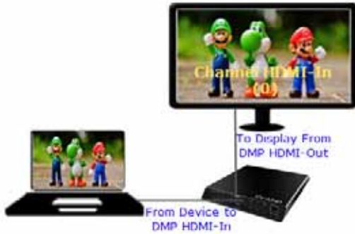
Figure 5 Local HDMI-In Pass-Through to Single TV Display
