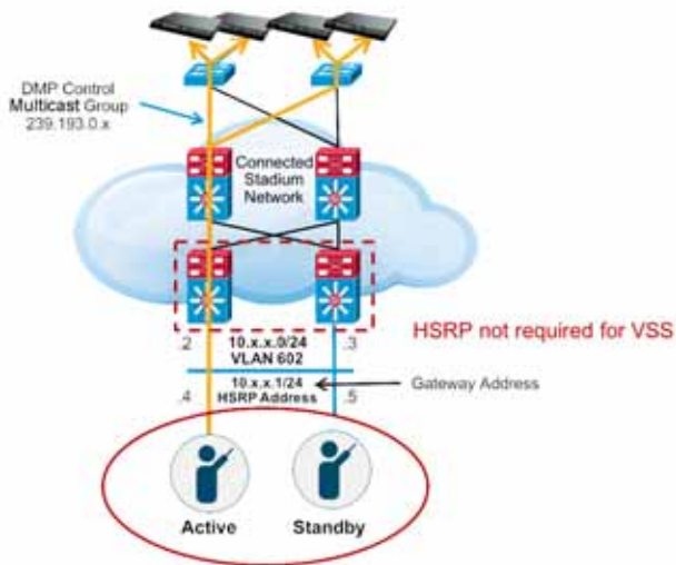
Figure 14 Cisco Vision Server Configuration Overview
