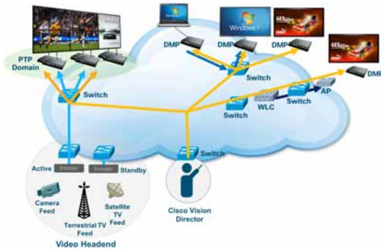
Figure 5 IP Multicast Overview
