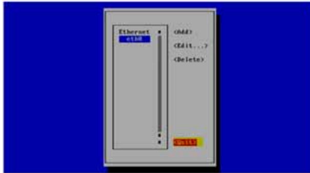
Figure 5 Exit Network Configuration TUI
