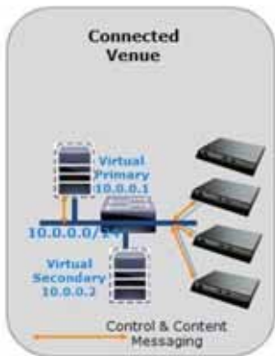
Figure 1 Cisco Vision Director Redundancy Under Normal Operation
