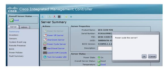
On the KVM Console/KVM terminal, confirm that the system is restarting and booting up from the Virtual CD/DVD.
