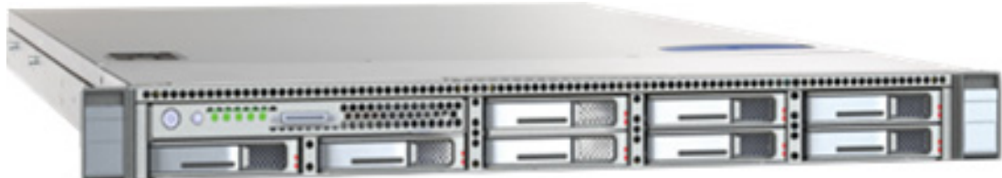
Figure 8 Front Panel of a Cisco UCS C220 M3 Rack Server
