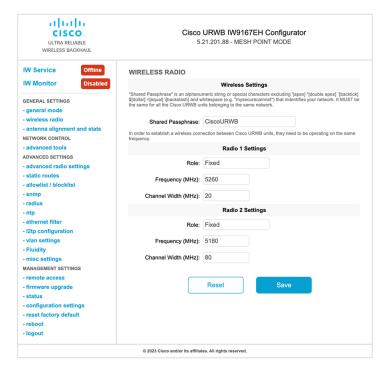
Following image shows the status of Radio channel and bandwidth configuration and specific information of each wireless interface.
