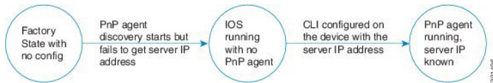
Figure 4: State Diagram for PnP Trigger with CLI Configured PnP Profile
