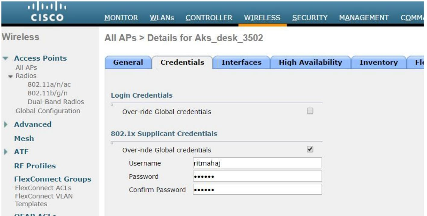
You can also set a common username and password for all the access points that are joined to the WLC with the Global Configuration menu.
