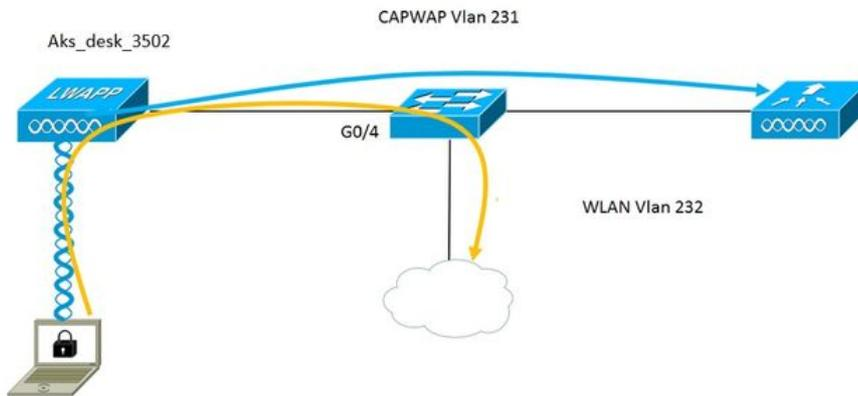
In this setup the access point acts as the 802.1x supplicant and is authenticated by the switch against ISE using EAP-FAST. Once the port is configured for 802.1x authentication, the switch does not allow any traffic other than 802.1x traffic to pass through the port until the device connected to the port authenticates successfully.
