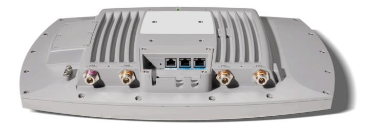
Any supported SIA antenna can be attached to the four N-Type connectors at the rear of the 9179F, note that only the left-most port is SIA capable. A dedicated 6dBi mini-patch antenna is available specifically for this purpose. The CW-ANT-T-D3-N is a dual-band 2.4GHz and 5GHz antenna with a  $90^{\circ}\times60^{\circ}$  (Azimuth  $\times$  Elevation) beamwidth in 5GHz and  $125^{\circ}\times60^{\circ}$  (Azimuth  $\times$  Elevation) beamwidth in 2.4GHz.
