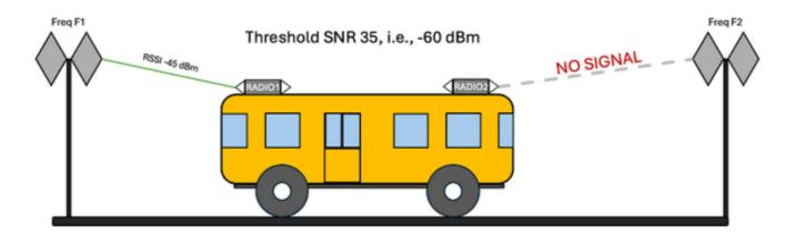
• In this example, while Radio 1 maintains a wireless signal of -45 dBm, Radio 2 detects a signal of -65 dBm from Trackside B, which is lower than the threshold. Consequently, Radio 2 scans for a better signal. If Frequency Scan Periodic is configured, Radio 2, being idle, continues to scan for a better trackside connection.
