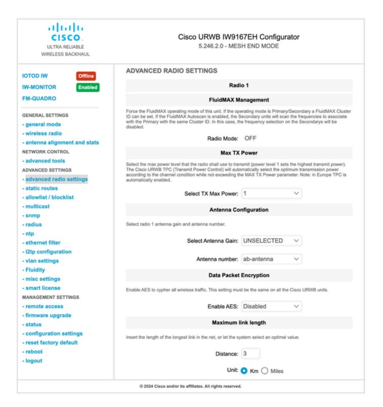
5. **Finalizing Configuration:** After configuring all settings, save the configuration and apply the changes. Once the Access Points (APs) reboot and the radios are back online, you can check the RSSI from the Antenna Alignment page and monitor live connectivity from the FM-Quadro page.
