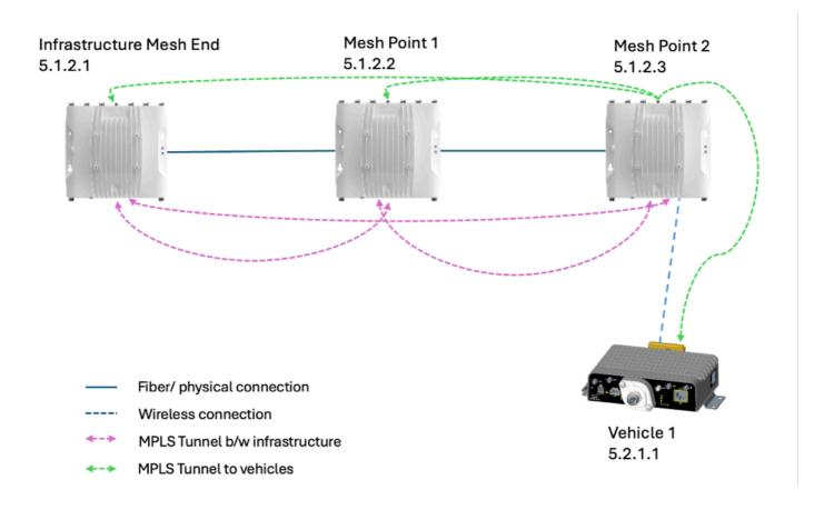
While LNO is disabled, check the **#show mpls config** output and you can see the pseudowires being built from all the Infrastructure radios to other Mesh points and the Mesh End. The psuedowires to vehicles are also built and not affected by LNO parameter.
