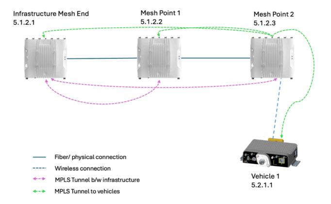
While LNO is enabled, check the **#show mpls config** output and you can see the pseudowires being built from all the Infrastructure Mesh points to only the Mesh End. The psuedowires to vehicles are also built and not affected by LNO parameter.
