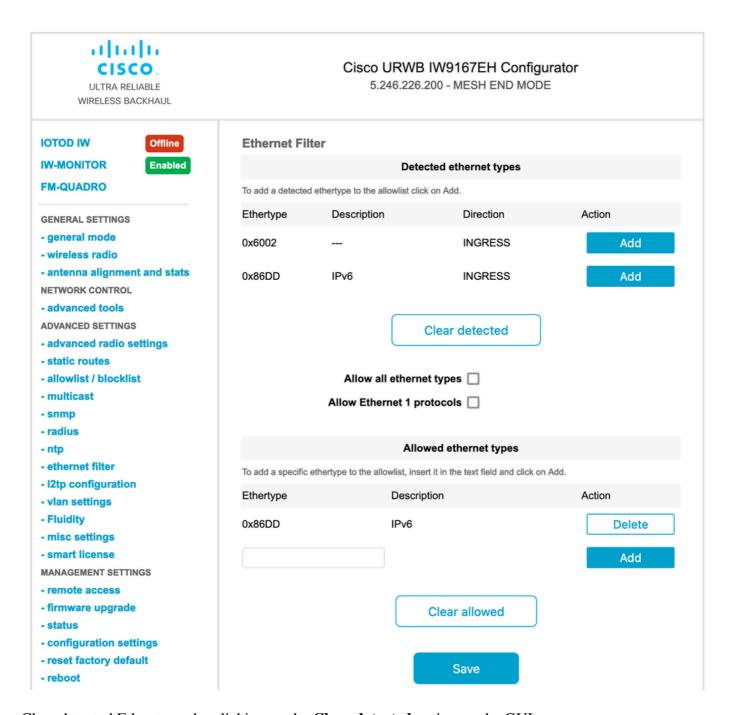
Clear detected Ether types by clicking on the Clear detected option on the GUI
