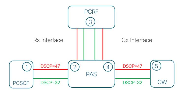
Two sets of peers are maintained between PCSCF, PAS, PCRF and GW. One set is configured to mark all IP packets with DSCP=32 (GREEN Set). while the other set marks all related IP packets with DSCP=47 (RED Set)
