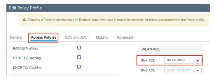
**Step 2** - Apply the ACL to the flex profile. Go to **Configuration > Tags & Profiles > Flex**, select the flex profile assigned to the flex connect APs. Under the **"Policy ACL"** section, add the ACL and click "Save"
