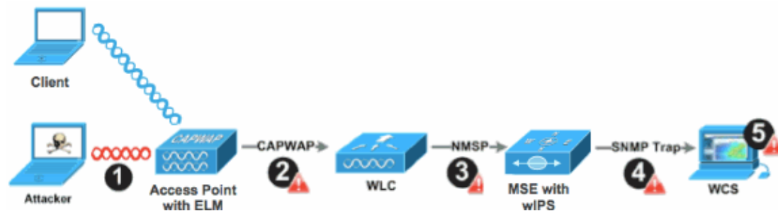
Figure 3 – Threat Detection and Alarm Flow
