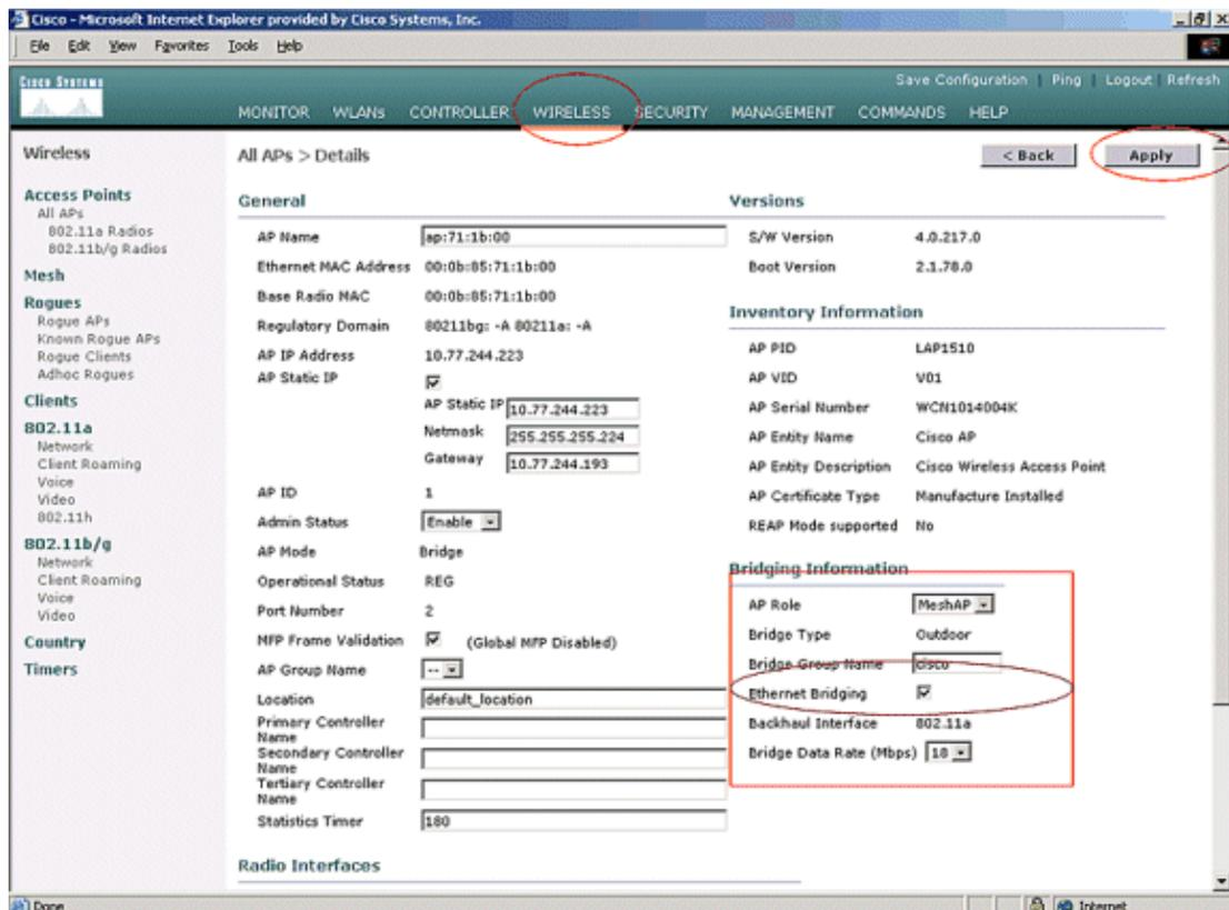
Once you finish the configurations of the bridge parameters and Ethernet bridging parameters on each AP, click **Apply** in order to save the settings. This causes the AP to unregister from the WLC, reboot, and reregister with the WLC.
