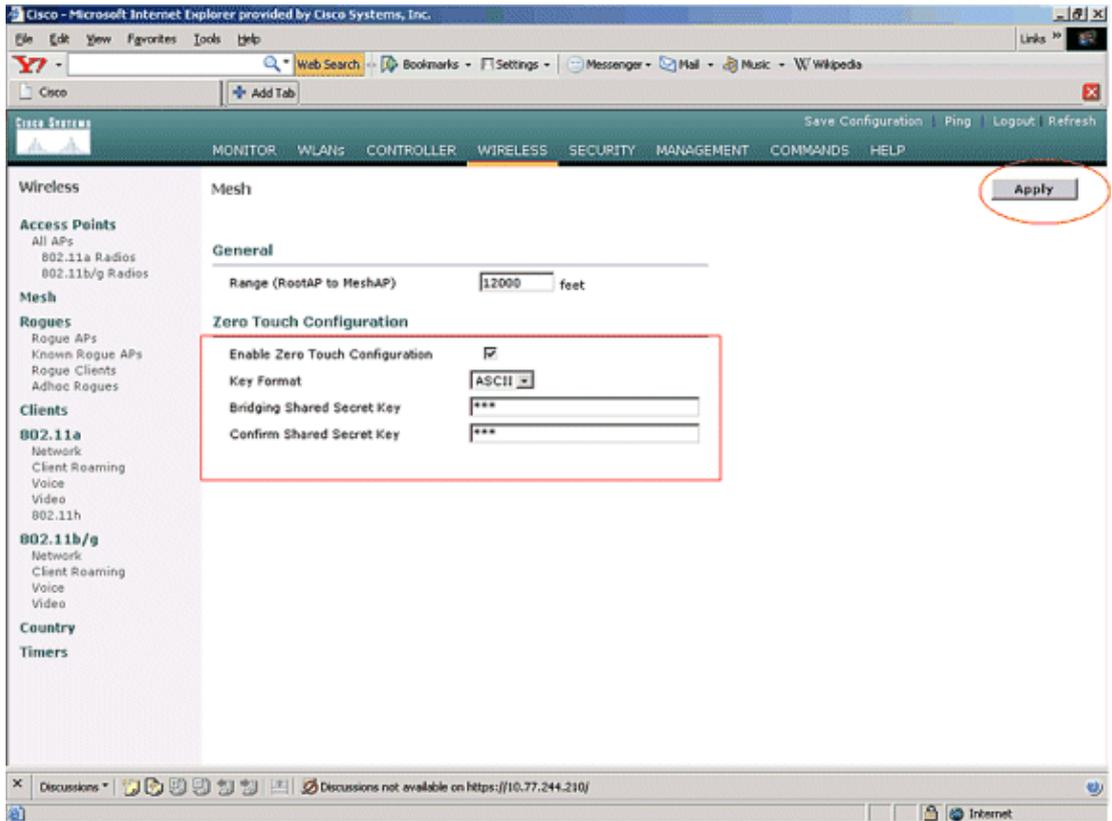
If zero-touch configuration is enabled on the Cisco wireless LAN controller and the MAP is moved to the other end of the mesh network, the RAP and MAPs do this to accomplish a secure zero-touch configuration:
