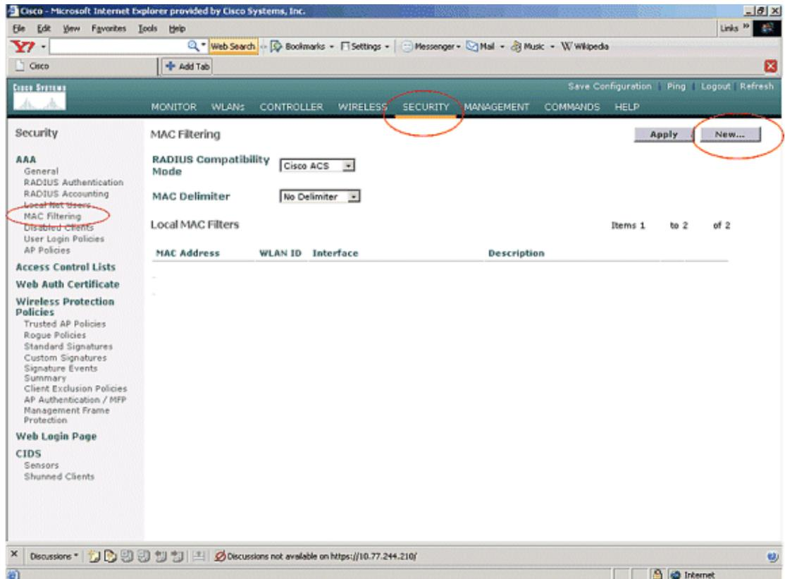
2. Enter the **MAC Address** of the AP and its **description** in the appropriate text boxes as given in this example. Also, choose a **WLAN** and **dynamic interface** from the WLAN ID and Interface Name drop-down menus, respectively. Click **Apply**.
