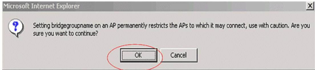
You can configure the bridge group name with the controller CLI with the command **config ap bridgegroupname set cisco** .
