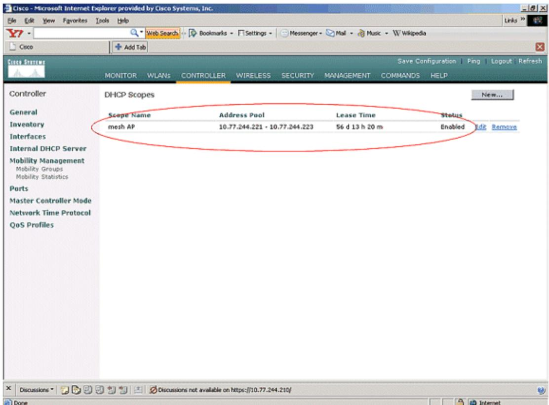
5. Once the APs are registered with the controller, assign the static IP address to the APs through the controller GUI. If you assign Static IP addresses to mesh APs, it provides faster convergence of the APs the next time they register with the controller.
