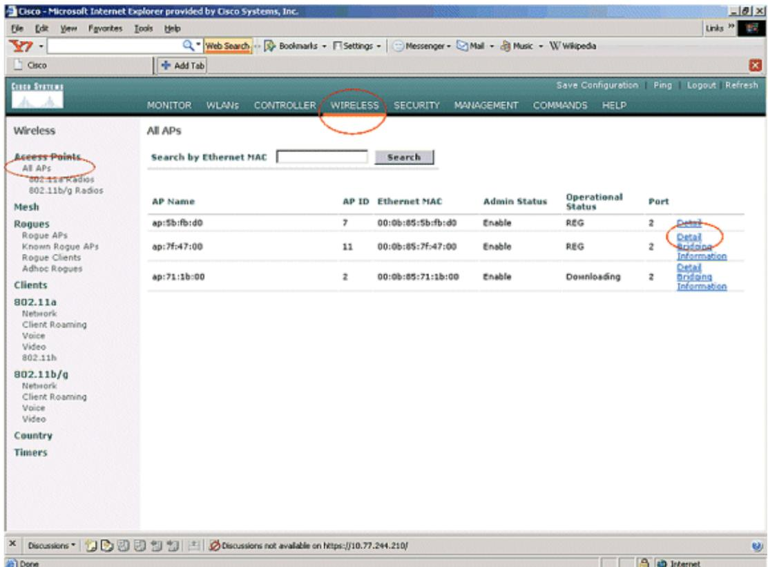
3. Under **Bridging Information**, check the box next to **Ethernet Bridging**. This enables Ethernet bridging on the AP.
