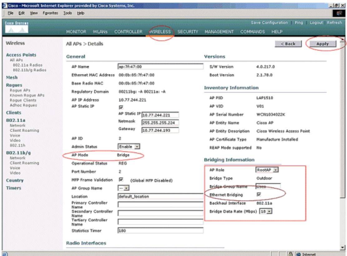
If you use a point to multipoint mesh network, enable the Ethernet bridging on the RAPs and only on the MAPs to which Ethernet devices are connected. It is not necessary to enable Ethernet bridging on all MAPs in a mesh network.
