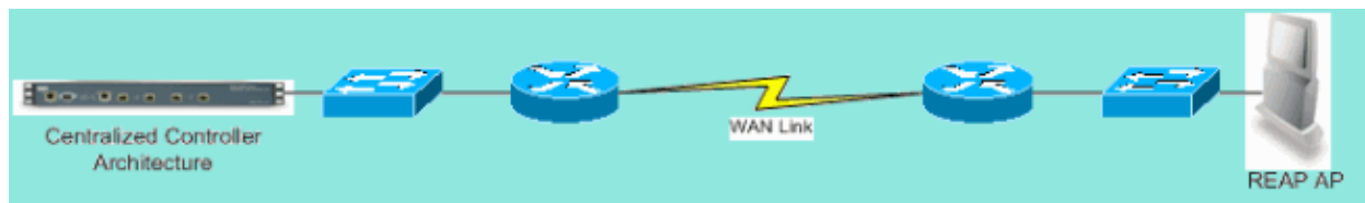
Figure 1: Basic REAP Architectural Diagram
