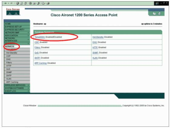
3. Click **Telnet/SSH** in order to enable and configure the Telnet/SSH parameters.
