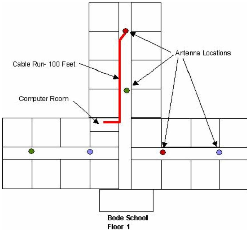
A coaxial cable carries radio frequency (RF) energy between the antennas and the radio equipment. An antenna cable introduces signal loss in the antenna system for both the transmitter and receiver. In order to reduce signal loss, minimize the cable length and use only low-loss (LL) or ultra low-loss (ULL) antenna cable in order to connect radio devices to antennas.
