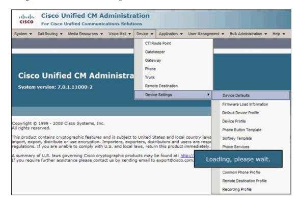
The Device Defaults Configuration list appears. This list shows the firmware that the IP Phone will load when it registers with CUCM. In this example, the Cisco 7961 IP Phone will load SCCP41.8–4–1S when it register with the Cisco Unified Communications Manager.
