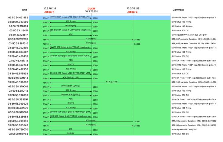
8. If any of the SIP messages is of interest for the investigation click the message and Wireshark automatically highlights the message in the packet capture. You can then perform a deep inspection to that specific packet. Expand the Session Initiation Protocol information of concern here, which is found in the packet details.
