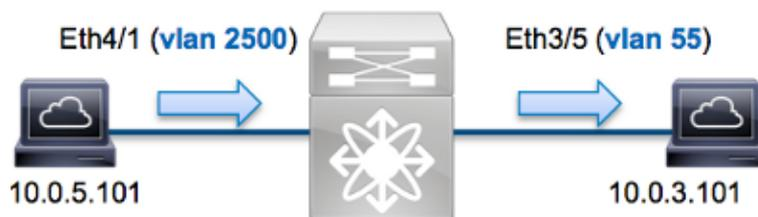
In this example, a host on VLAN 2500 (**10.0.5.101**), port **Eth4/1** sends an Internet Control Message Protocol (ICMP) request to a host on VLAN 55 (**10.0.3.101**), port **Eth3/5**. ELAM is used in order to capture this single packet from **10.0.5.101** to **10.0.3.101**. It is important to remember that ELAM allows you to capture a single frame.
