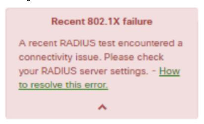
A test is considered successful if the Meraki device receives any legitimate RADIUS response (Access-Accept/Reject/Challenge) from the server.
