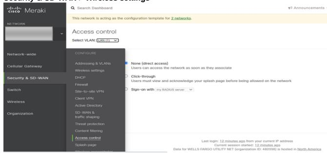
2. MR-Access points (enabled on a per Service Set Identifier (SSID) basis): Wireless > Access control
