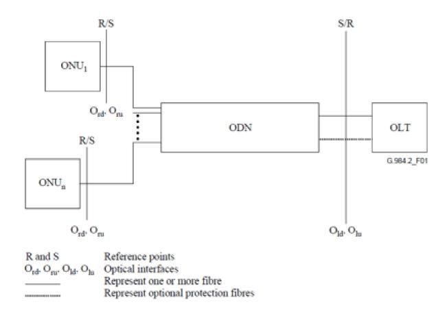
• The OLT is connected to the optical splitter through a single optical fiber, and then the optical splitter connects to ONUs/ONTs.
