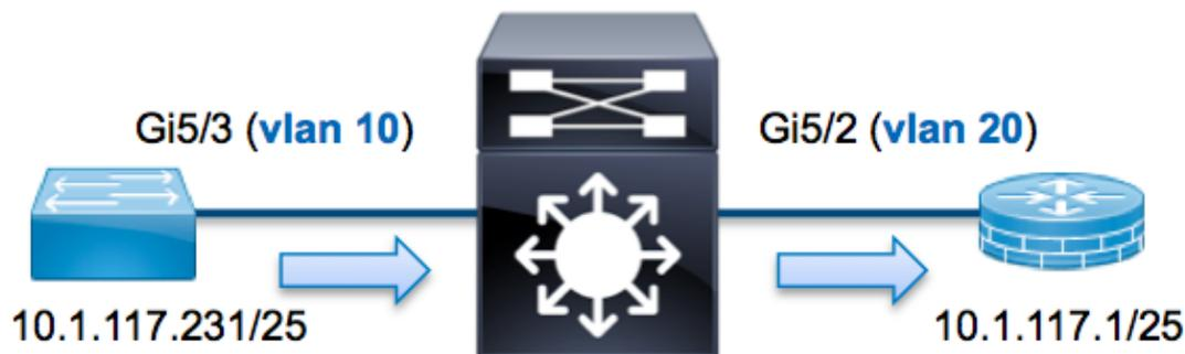
In this example, a host on VLAN 10 (*10.1.117.231*), port *G5/3* sends an Internet Control Message Protocol (ICMP) request to a host on VLAN 20 (*10.1.117.1*), port *G5/2*. ELAM is used in order to capture this single packet from *10.1.117.231* to *10.1.117.1*. It is important to remember that ELAM allows you to capture a single frame.
