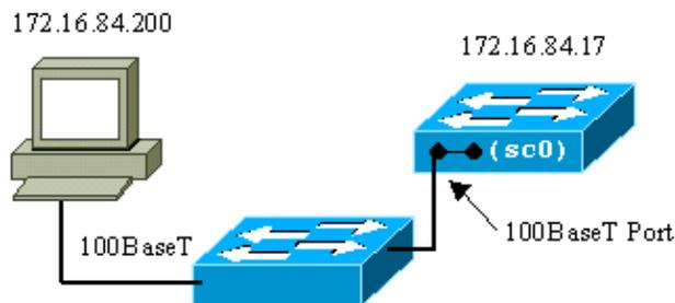
The me1 is actually a physical Ethernet port on the Supervisor Engine module on the Catalyst 4500/4000 series switches. This interface is used for network management only and does not support network switching.
