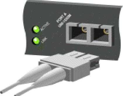
This is used in order to connect to 100Base-FX fiber-optic ports. Use multimode fiber (MMF) cables with MT-RJ connectors.
