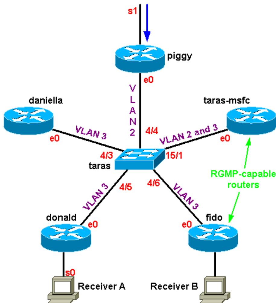
In this case, only fido and the Multilayer Switch Feature Card (MSFC) in taras are RGMP-capable routers; donald, daniella, and piggy are non-RGMP-capable routers. There is a multicast source 4.4.4.1 sending to 224.1.1.1 located on the serial behind piggy. Taras-msfc is doing the Inter-VLAN routing between VLAN 2 and VLAN 3. There is no receiver in VLAN 2 but two receivers in VLAN 3: one behind fido and one behind donald.
