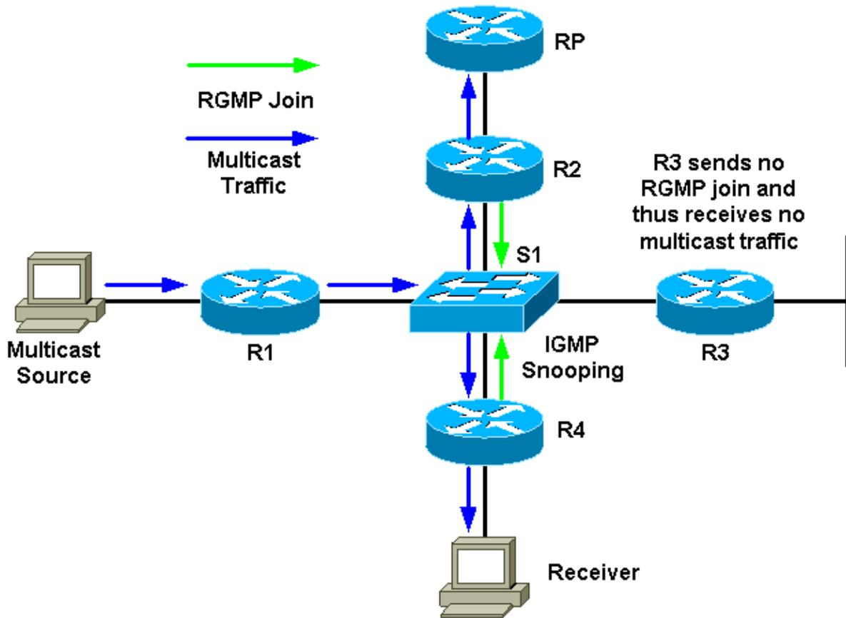
R2 and R4 will send an RGMP join for that multicast group to the switch. R3 will not send an RGMP join. As a result, the switch will only forward the multicast traffic received from R1 for that group to R2 and R4 and not to R3. This decreases traffic on the network.
