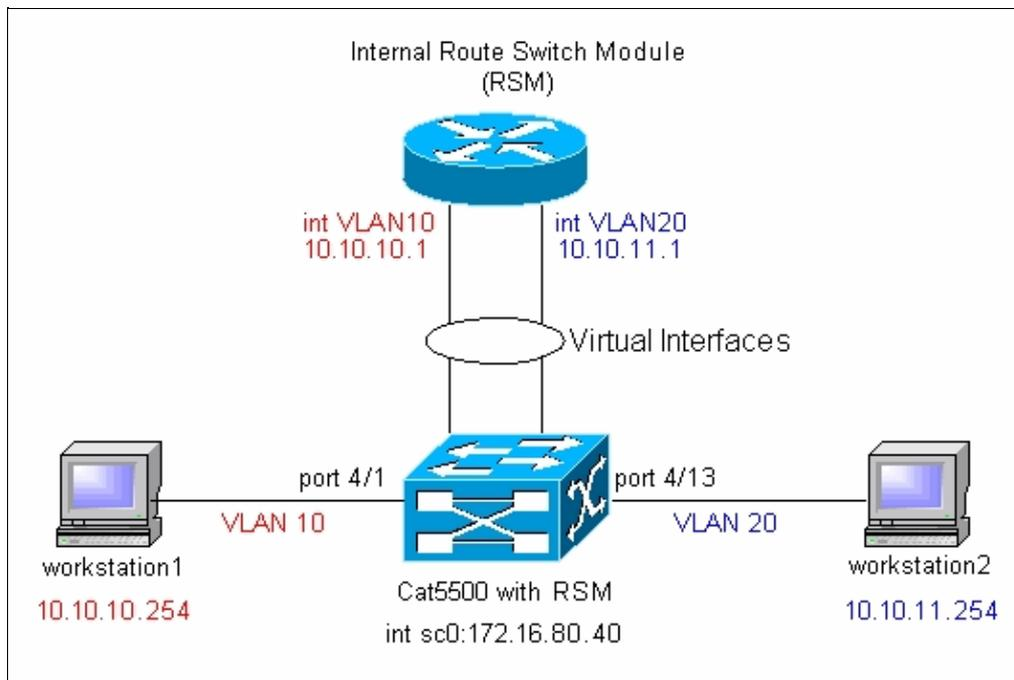
**Note:** Do not connect workstation1 and workstation2 unless you are asked to do so in this document. This document points out a common problem that customers report when they configure interVLAN routing or multiple VLAN interfaces on the router module. See the Common Issue: VLAN Interface Shows down/down section for details.
