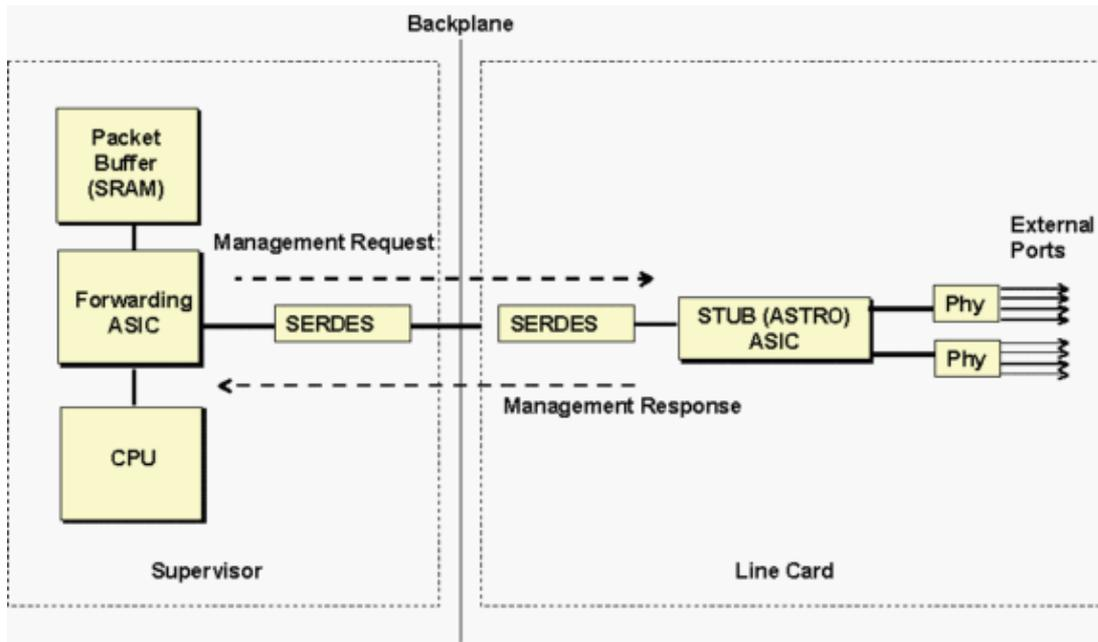
The Supervisors communicate to the Line Card stub ASIC through the SERDES (SERializer–DESerializer) component. There is a SERDES component on the Supervisor side connecting to the backplane and another SERDES on the line card for each stub ASIC for connecting to the backplane.
