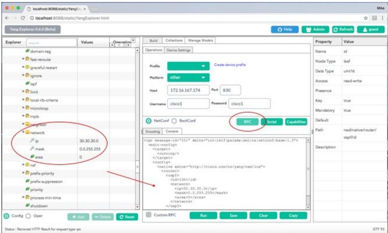
Next, **Run** is selected in order to send the RPC message to the Catalyst 3850 via NETCONF. The Catalyst 3850 replies back with an ok message to let the user know the operation was successful.
