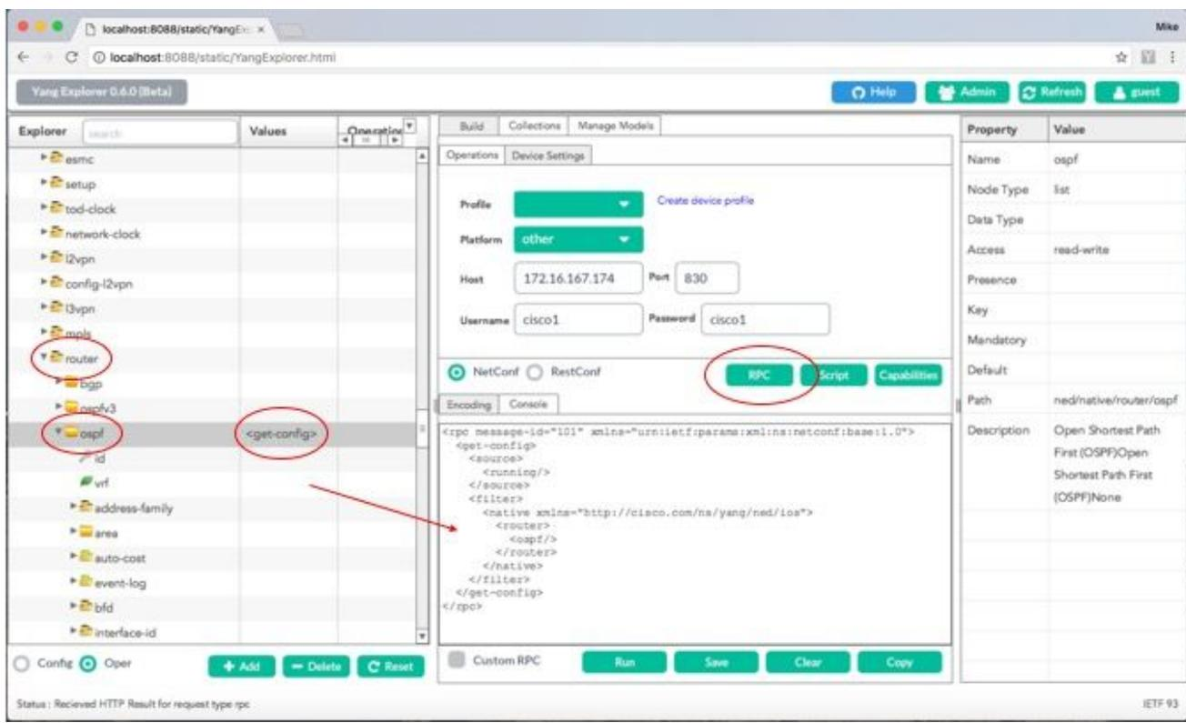
Next, **Run** is selected in order to send the RPC message to the Catalyst 3850 via NETCONF. The Catalyst 3850 replies back with its OSPF routing configuration.
