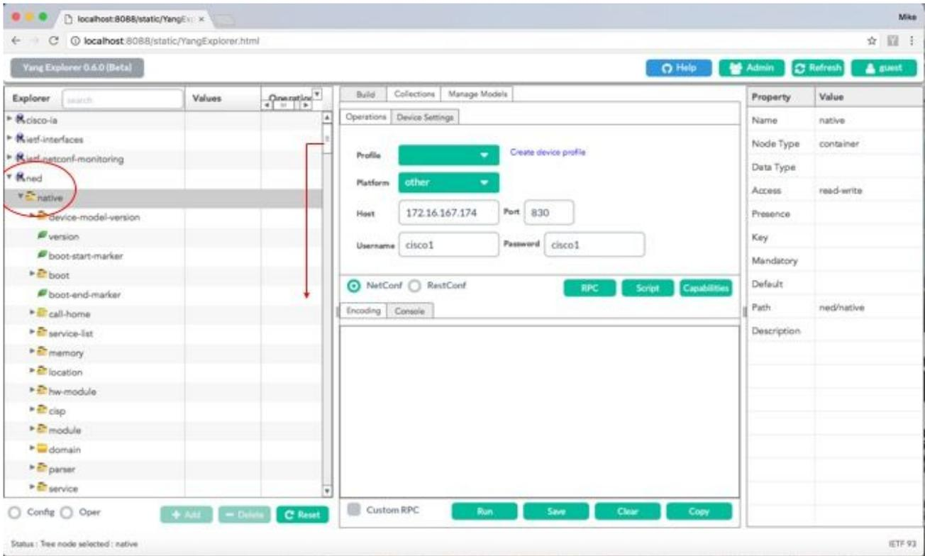
As an example, these screenshots demonstrate how to display the OSPF routing configuration of the Catalyst 3850 after first scrolling down the list of available ned.yang data model configuration options in the Explorer section on the left side of the YANG Explorer application GUI. The ospf sub-option is located inside of the router option. The associated get-config RPC is generated when you select the **RPC** button.
