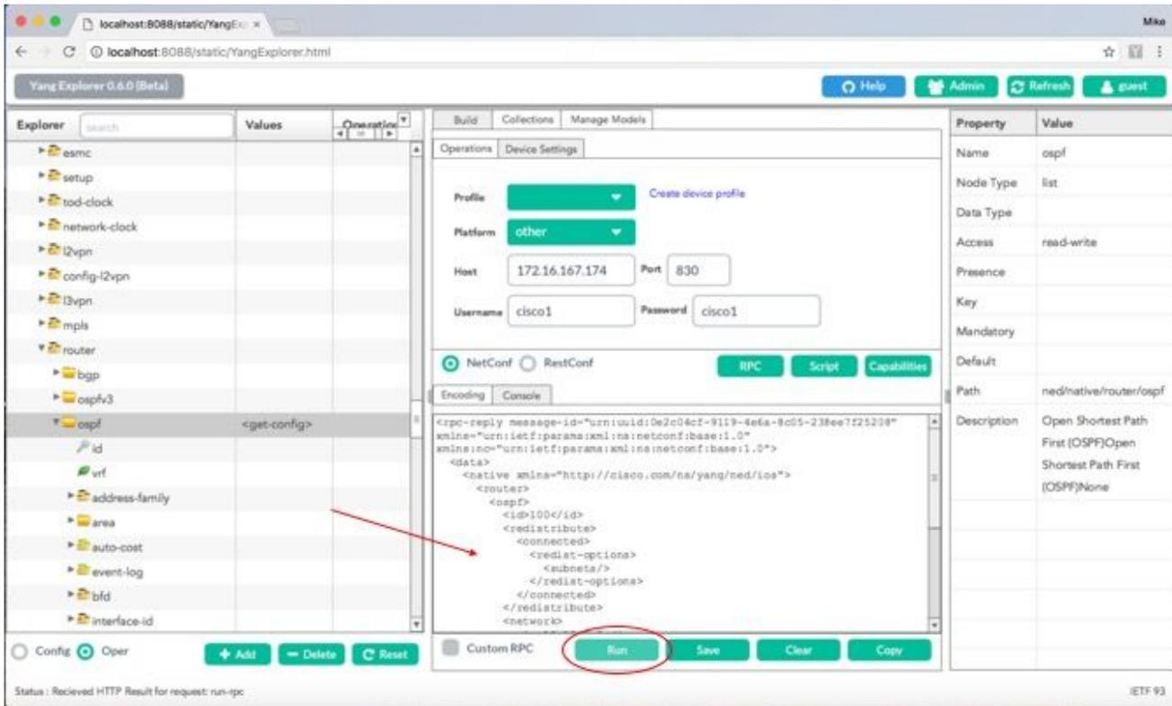
Here is an expansion of the OSPF routing configuration returned by the Catalyst 3850 in response to the get-config RPC operation.
