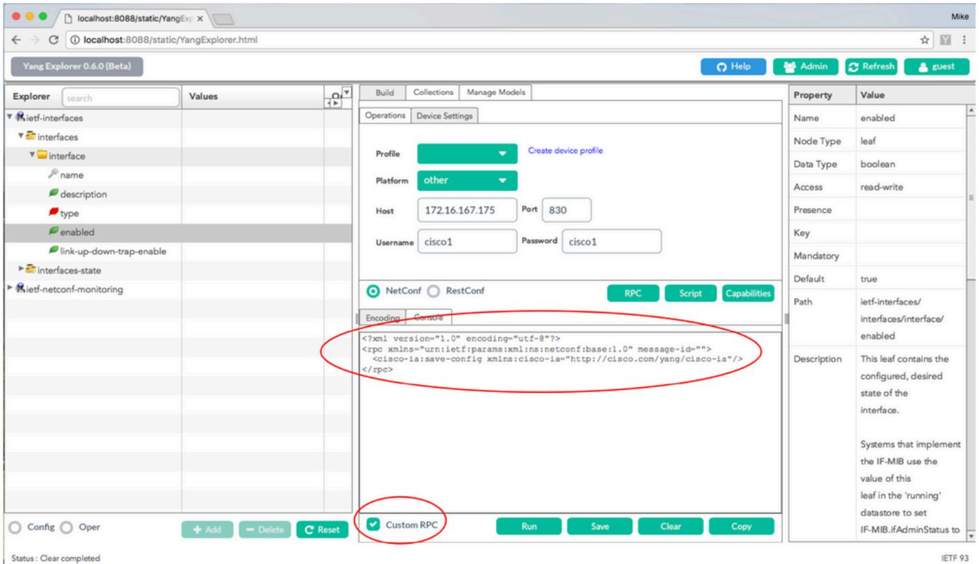
**Run** is selected in order to send the custom RPC message to the Catalyst 3850 via NETCONF. The Catalyst 3850 replies back with a successful message.
