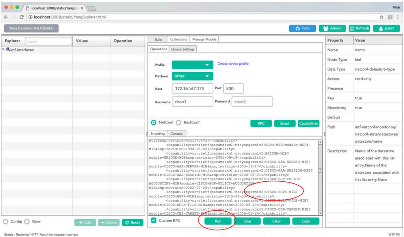
Option 3. A list of available MIB models can be viewed in the NETCONF capabilities and Hello message returned by the Catalyst 3850 in response to an SSH connection from the Centralized Management Platform (Laptop).
