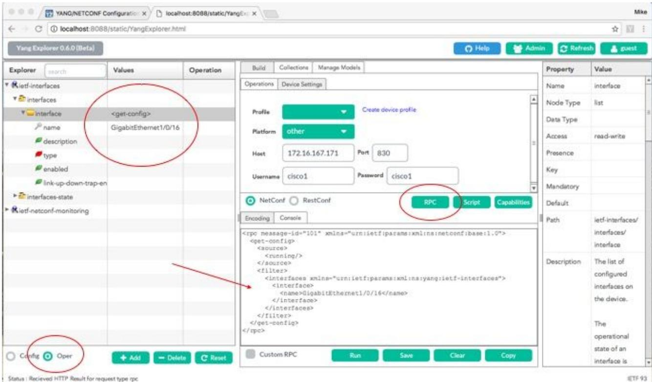
**Run** is selected in order to send the RPC get-config message for GigabitEthernet1/0/16 to the Catalyst 3850 via NETCONF. The Catalyst 3850 replies back with the GigabitEthernet1/0/16 interface configuration which shows enabled = true.
