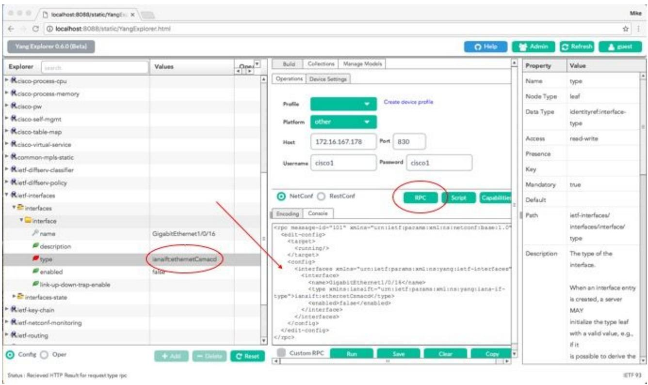
This time, once **Run** is selected to send the RPC message to the Catalyst 3850, the Catalyst 3850 replies with an ok message to indicate that the operation was successful.
