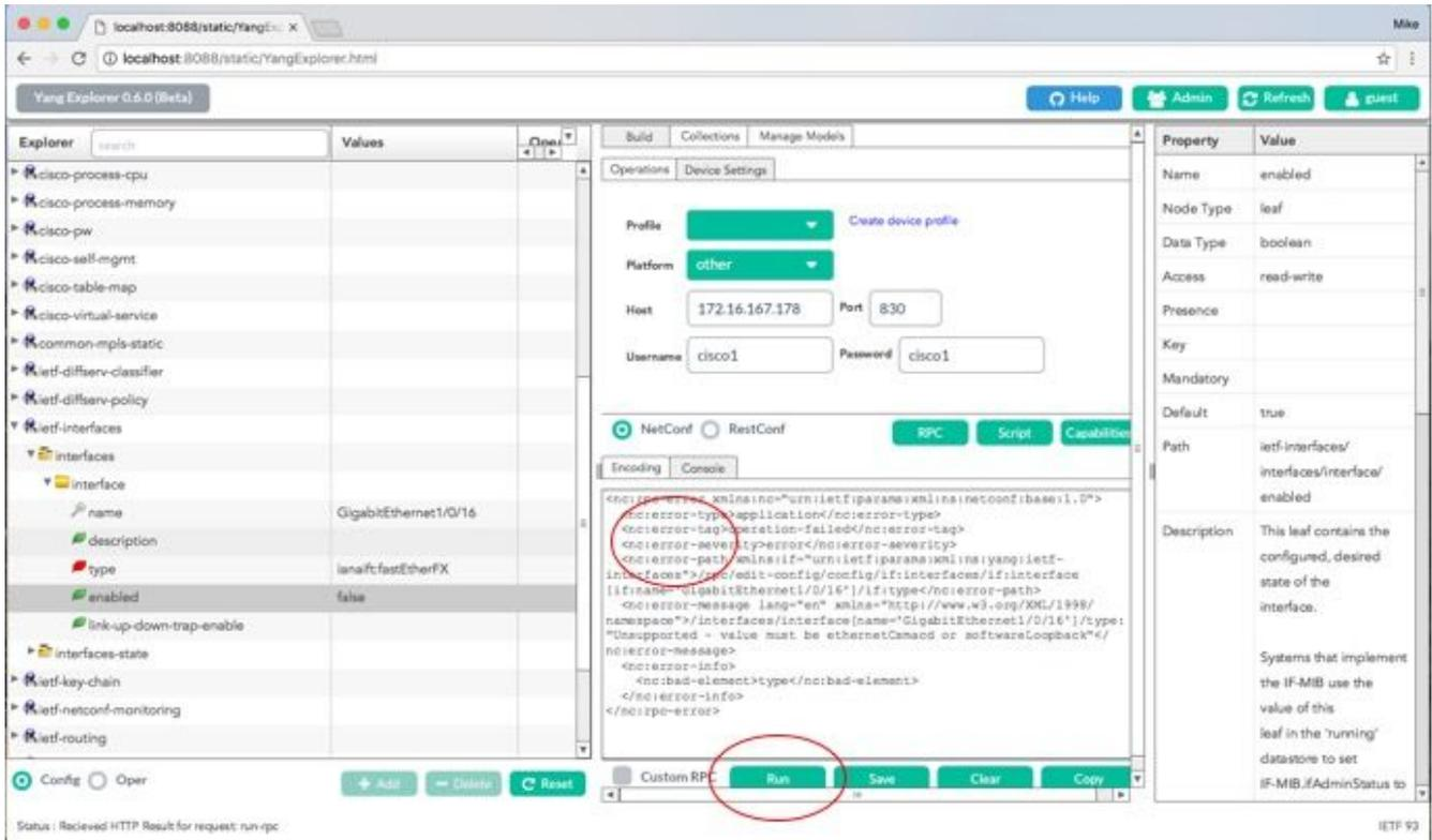
Here is the error that was returned by the Catalyst 3850. Notice that it contains an error tag “operation-failed” and further detail that concerns the error says “Unsupported - value must be ethernetCsmacd or softwareLoopback”</nc:error-message>”.
