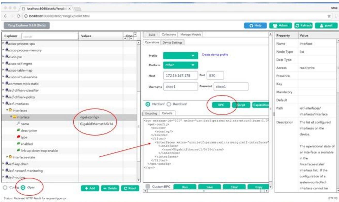
Once **Run** is selected to send the RPC message to the Catalyst 3850, the Catalyst 3850 replies with the YANG formatted interface configuration which shows that interface type is ianaif:ethernetCsmacd.
