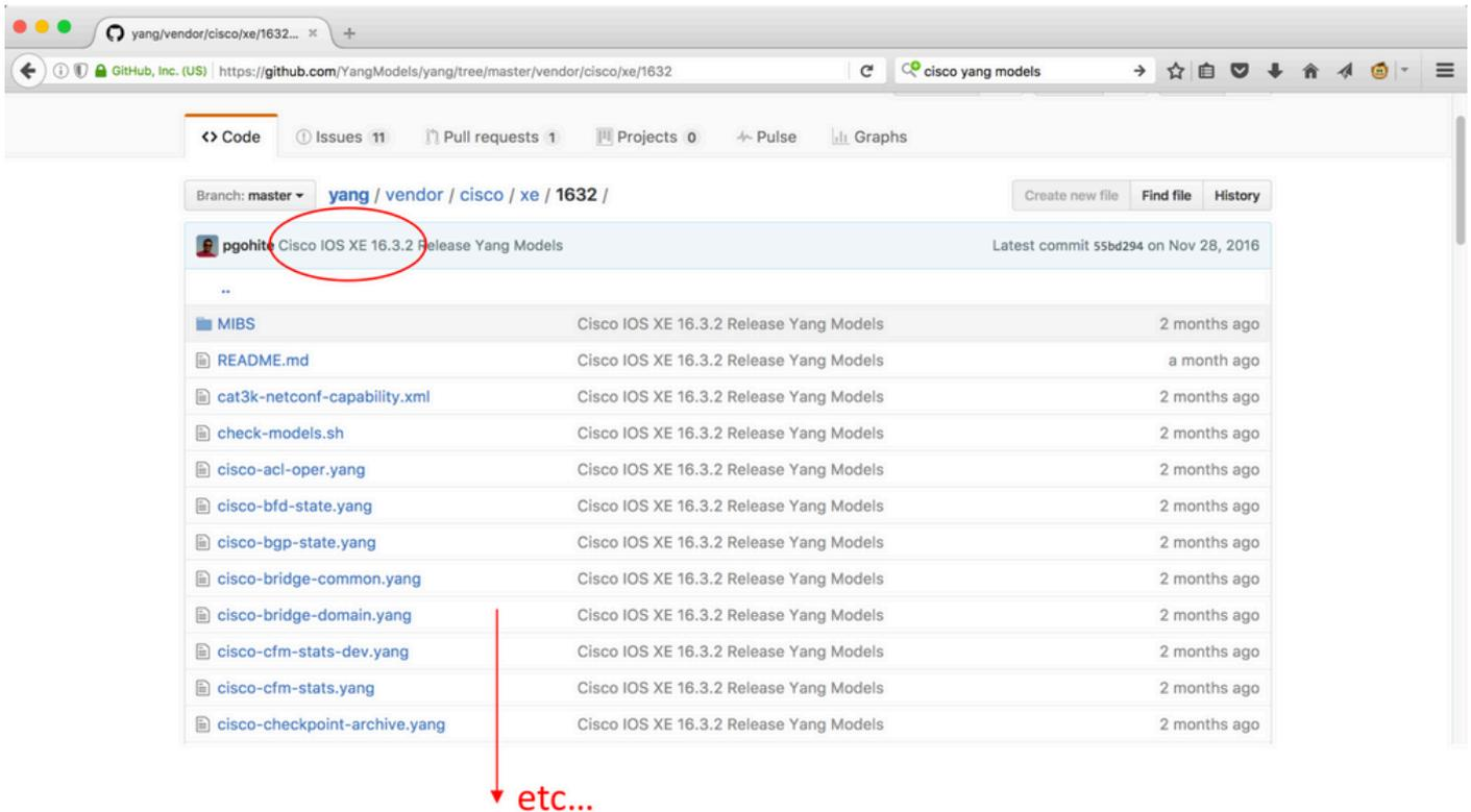
These files can be downloaded onto the Centralized Management Platform (laptop) and then, in turn loaded into the Yang Explorer application. There are two ways to do this. The first is to load in the various YANG data model files individually, the second is a bulk loading of all the files.
