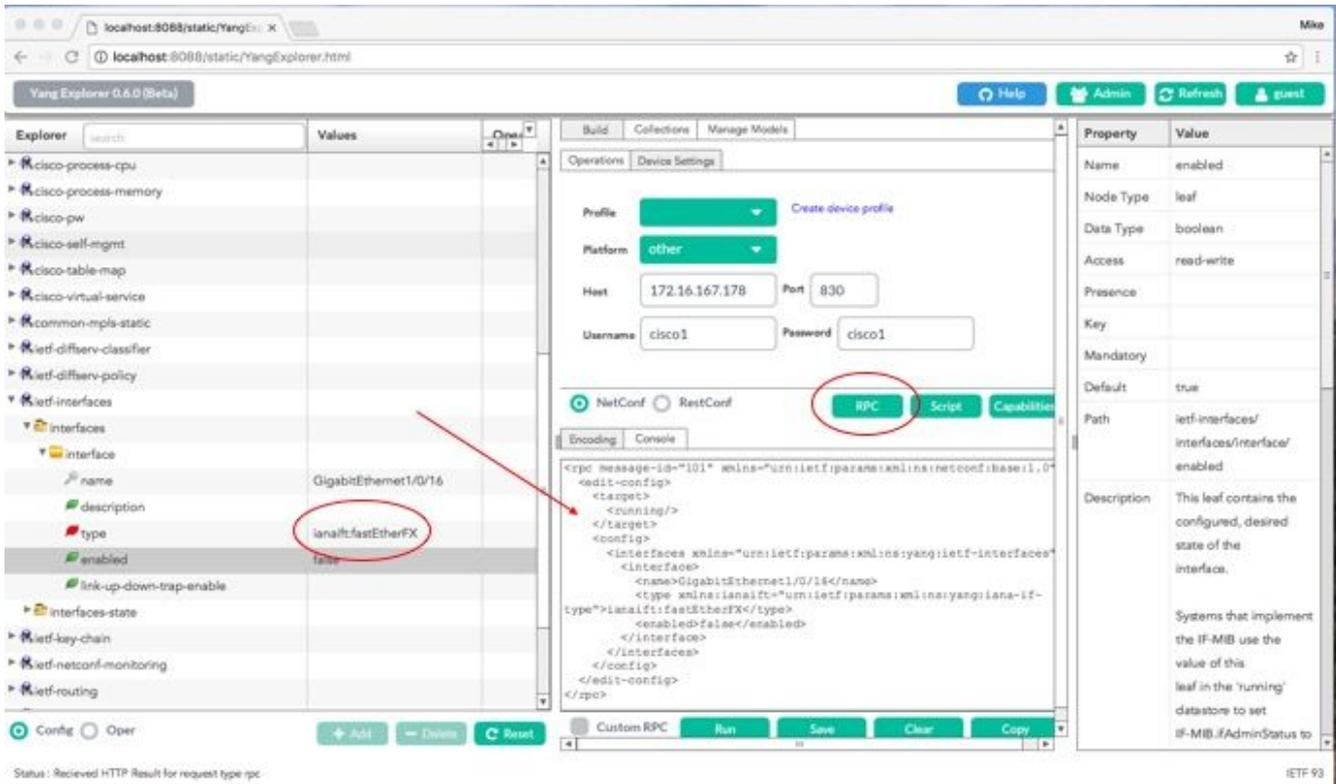
Once **Run** is selected to send the RPC message to the Catalyst 3850, the Catalyst 3850 replies with an error message.
