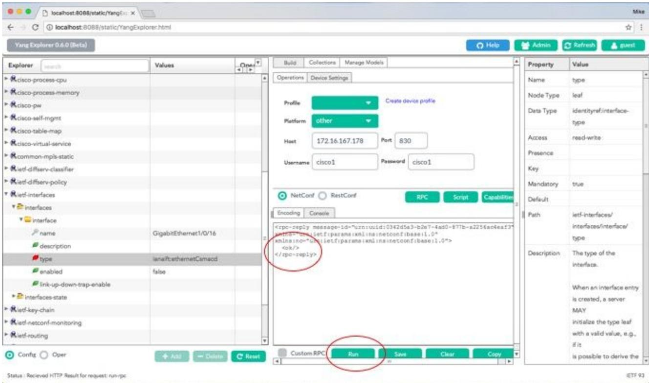
**Tip:** When unsure what the correct Explorer Values format can be, the configuration that exists can be looked at before you attempt to make a change to it's parameters. This can be done with the **get-config** operation (Oper) as shown.
