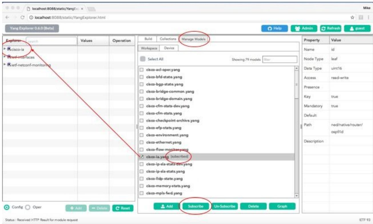
Once the cisco-ia data model is expanded in the Explorer section on the left of the YANG Explorer application GUI, the various operational options are seen. As an example, to use one of the available cisco-ia.yang data model options, the **save-config** operation is selected and the associated RPC is generated when you select the **RPC button**.
