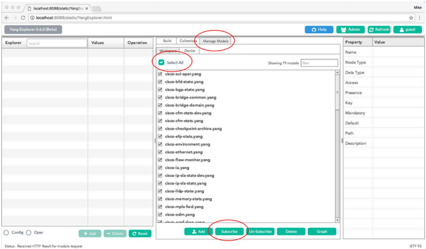
The screenshot shows the Yang Explorer 0.6.0 (Beta) interface. The 'Manage Models' tab is active, displaying a list of 79 models. The 'Select All' checkbox is checked, and the 'Subscribe' button is highlighted with a red circle. The interface includes a search bar, a table of models, and a 'Property Value' table on the right.
