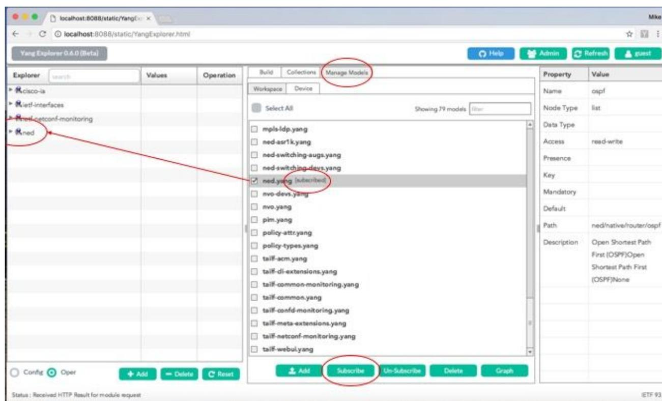
Scrolling through the available options in the Explorer section on the left side of the YANG Explorer application, GUI shows a long list of configurable Catalyst 3850 features in the ned.yang data model.
