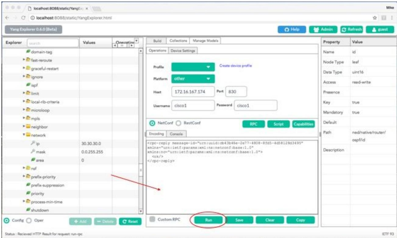
This NETCONF/YANG RPC operation to modify the OSPF routing configuration via the ned.yang data model is reflected in the Catalyst 3850 configuration as seen via the Catalyst 3850's CLI. There is also a syslog message on the Catalyst 3850 that indicates that a configuration change was made via NETCONF.
