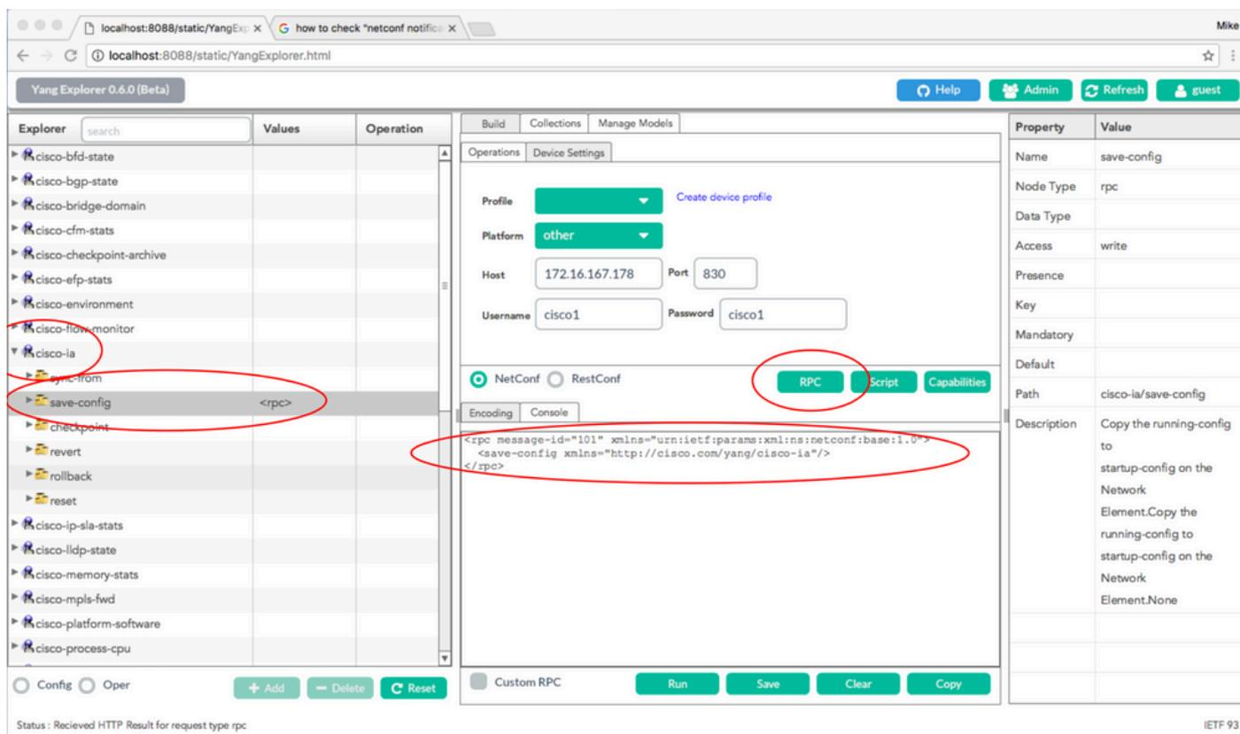
**Run** is selected to send the custom RPC message to the Catalyst 3850 via NETCONF. The Catalyst 3850 replies back with a successful message.
