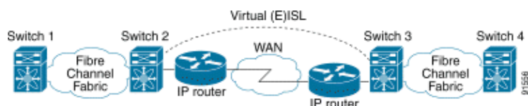
Figure 1 Fibre Channel SANs Connected by FCIP
