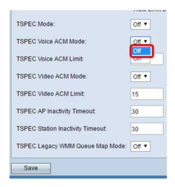
Step 15. Enter the maximum amount of traffic the WAP tries to transmit wirelessly with a voice admission control to gain access in the *TSPEC Voice ACM Limit* field.
