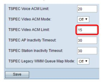
Step 18. Enter the amount of time in second for the WAP to detect a downlink traffic speculation as idle before the WAP deletes it in the *TSPEC AP Inactivity Timeout* field.
