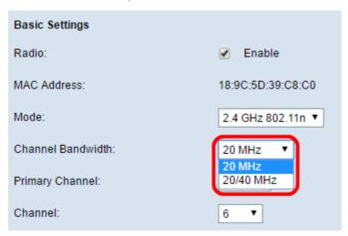
Step 7. From the Primary Channel drop-down list, choose a channel to set as primary. The primary channel is used for devices that only support 20/40 MHz channels. The options are:
