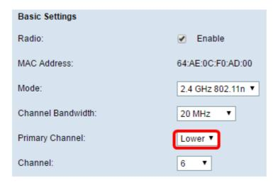
**Note:** The Primary Channel drop-down list is automatically disabled if the Channel Bandwidth is set to 20 MHz.
