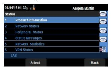
Step 3. Use the navigation keys and scroll down to Peripheral Status. Press the **Select** softkey. The *Peripheral Status* menu appears.
