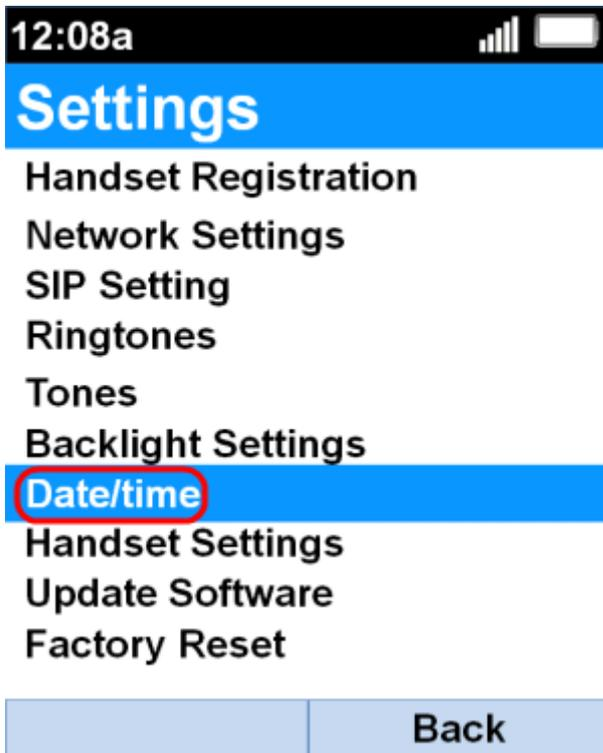
Step 2. On the *Settings* menu, choose **Date/time** with the use of **up** and **down** navigation buttons and press the **Select** button.
