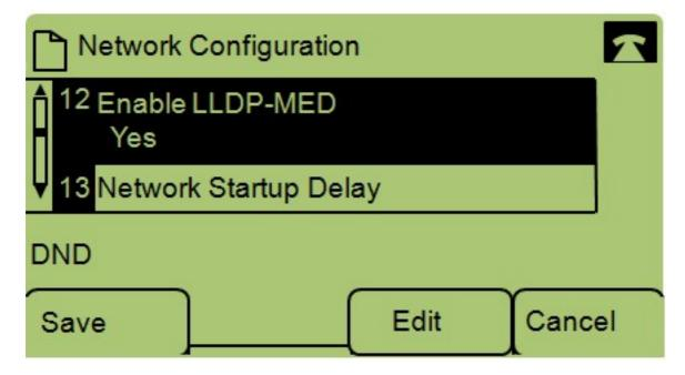
Step 4. Navigate to Enable LLDP-MED and press Select using the soft-key.
