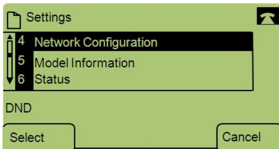
Step 3. Navigate to Network Configuration and press Select using the soft-key.
