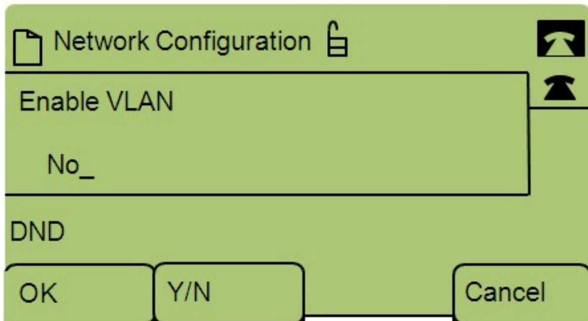
Step 6. Press **Y/N** to toggle between Yes and No to enable or disable the VLAN.
