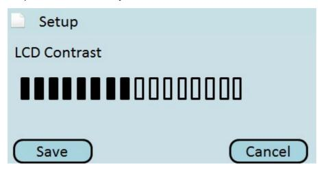
Step 2. Use the right and left navigation buttons to adjust the LCD contrast to an optimal level.
