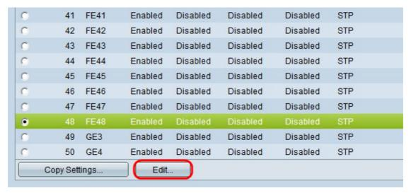
Step 4. Click the radio button of the port or LAG that is connected to the other switch and click **Edit**. The *Edit STP Interface* window appears:
