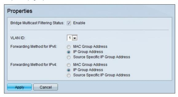
Step 2. Check **Enable** in the Bridge Multicast Filtering Status field to enable multicast filtering.
