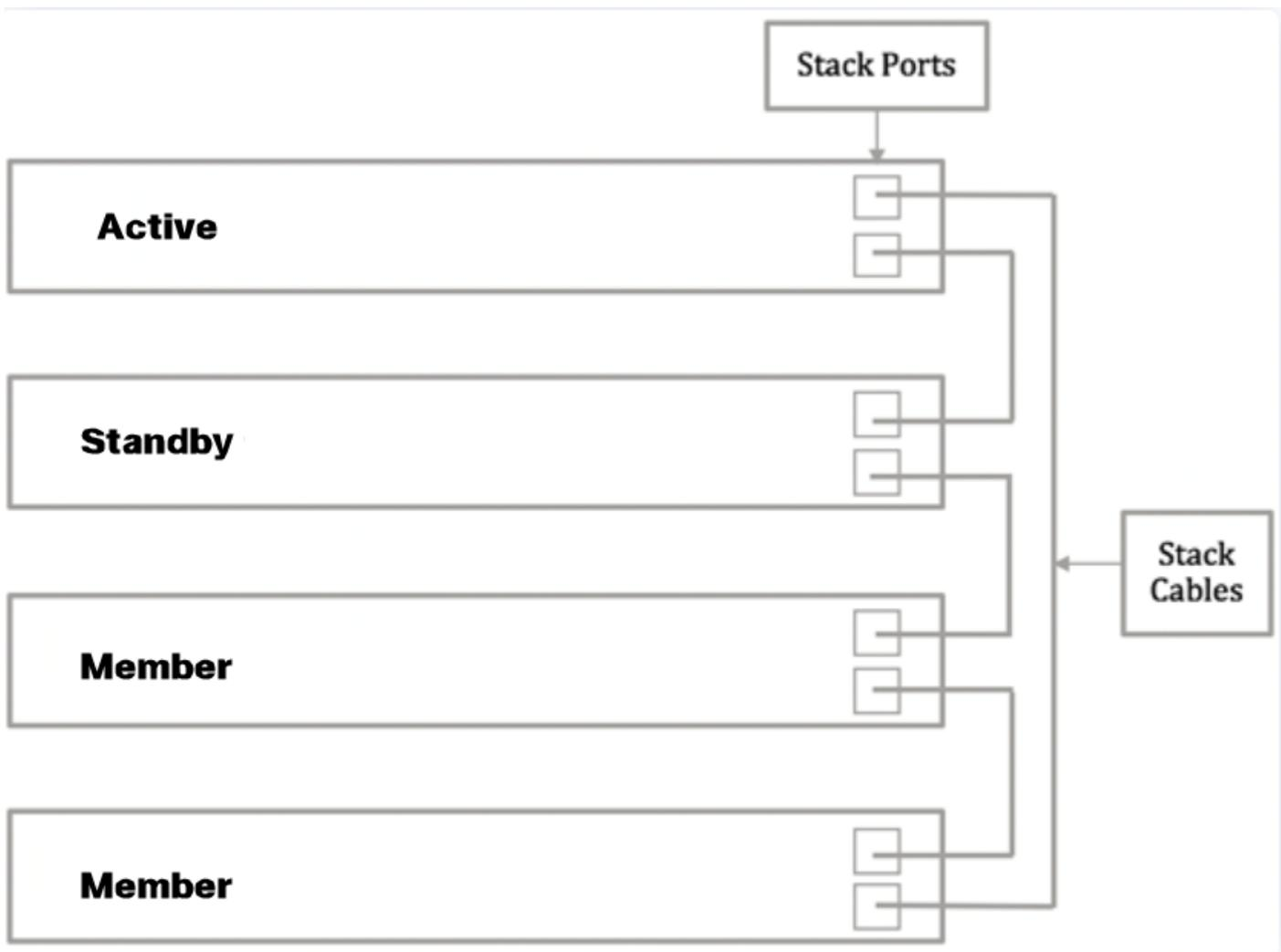
Step 2. Connect one end of the Small Form-Factor Pluggable (SFP) cable that came with your device into the SFP+, XG3, or XG4 port of your switch.
