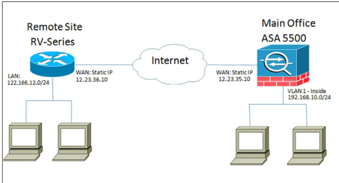
With this configuration a host in the remote site network of 122.166.12.x and a host in VLAN 1 at the main office can communicate with each other securely.
